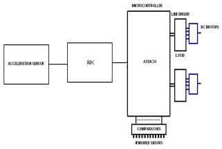
Fig 7: Block diagram automated wheelchair Working principle:
